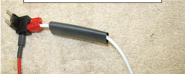
Slip back or carefully cut the shrink wrap that covers the fuse and spade. This will expose the 10A fuse and the tap at the end of the white wire.
