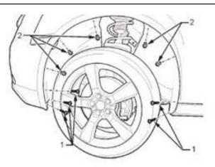
5. Remove the front wheel well liner by removing three screws in the front and two screws from the rear of the liner (1). Use a trim release tool to remove five scrivets (2) and remove the liner. Repeat steps on the RHS of the vehicle
