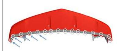
Remove the under carriage rubber seal located at the end of the fascia. Save the clips and seal. These will be reinstalled once the T5 splitter is mounted.
