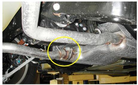
Figure 2: Driver's side nut removal
