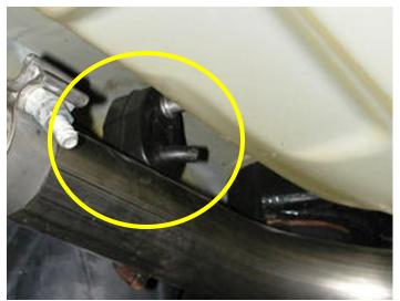
Figure 6: Stock rubber isolater
