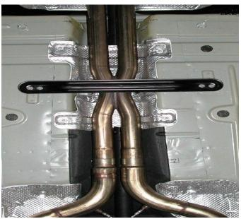
Figure 3: SLP X-pipe on factory downpipes
