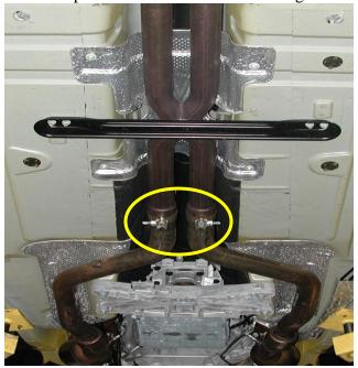
Figure 1: Loosen clamps
