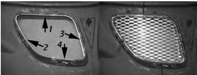
Fig. 4 - Sequence for fastening upper grille
