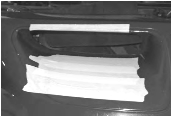
Figure 4. Mask off the upper opening to protect paint and make it easier to mark the hole locations.
