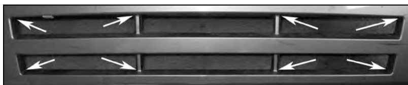
Figure 7. Locations to drill holes for lower grille option
