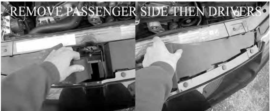
Figure 1. Begin by removing radiator cover.
