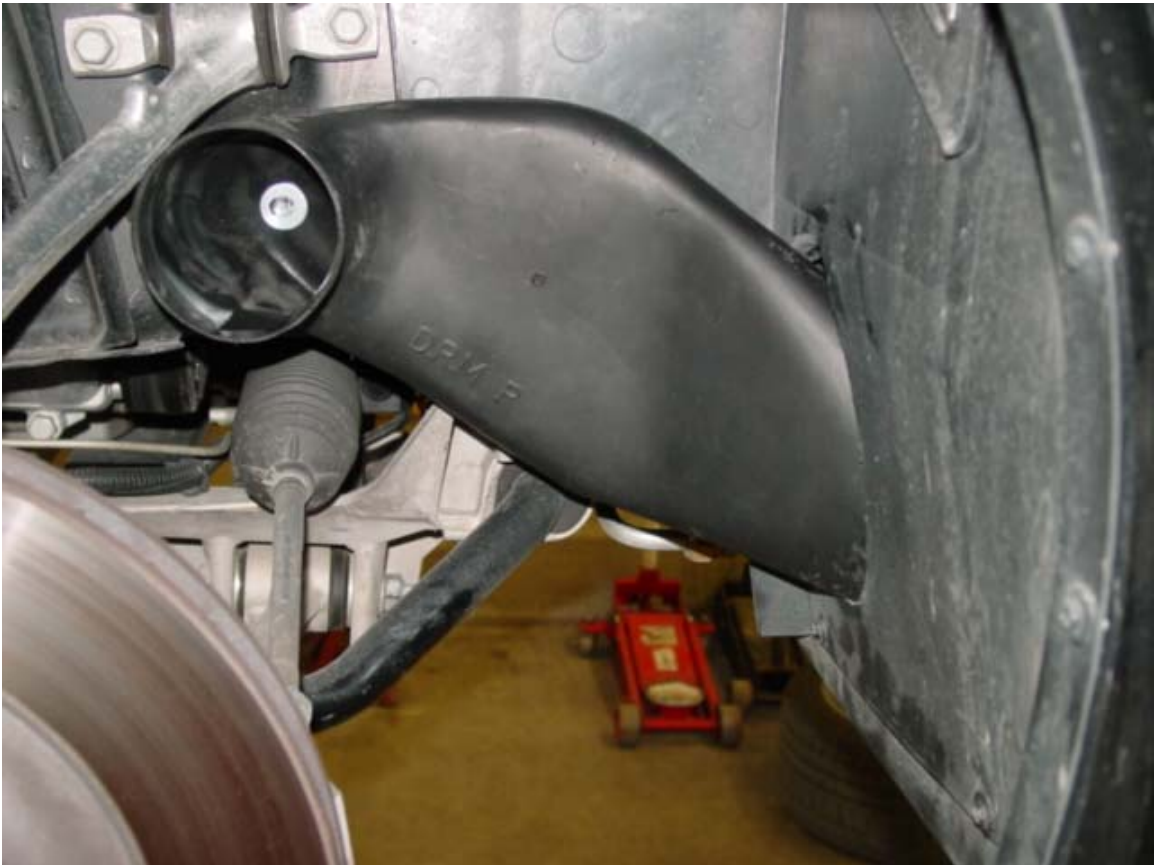
Screw location to mount the brake duct. Place the screw/washer through brake duct outlet after trial fit and drilling pilothole. (as pictured above)
