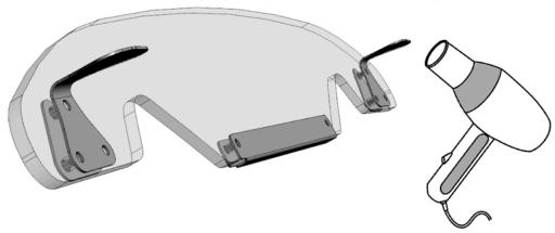
**Step-4** Center the windblocker from left to right on the panel then press firmly to mount. The two screws on steel bar (A) should perfectly line up with the two indentions on tonneau cover. (B) After confirming the product is centered apply firm pressure to both the front side of bracket and top side of bracket for 20 seconds. If you have the LED lighted version proceed to step 5. If you do not have the lighted version you are now finished!
