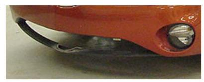
While double stick tape is already installed on the air dam, your shop should also use an adhesive to provide additional strength and durability. The double stick tape is not strong enough to hold the air dam in place by itself. Once installed, one sheet metal screw should be used in each wheel well where arrow is in picture at right.
