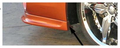
To prevent dirt from getting between the air dam and bumper, use a silicone caulking type of material across the top of the air dam where it meets the bumper all the way from the inside of the wheel well, across the front to the other wheel well. We used 3M super silicone sealant. Part number 05113508662 is black and part number 05113508661 is clear.
