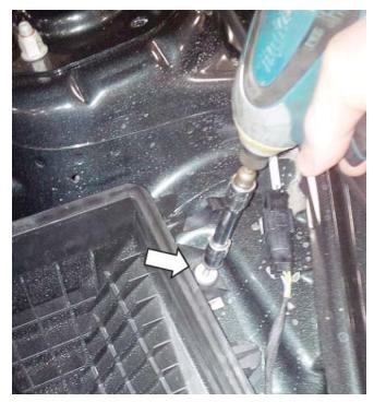
7. Remove the air box tray and dirty air inlet from the vehicle.
