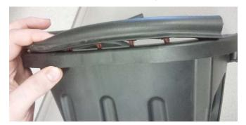
6. Insert the air box assembly into the vehicle.
