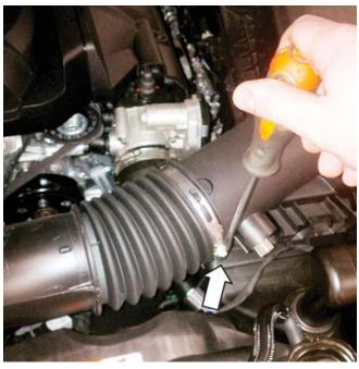
4. Release the two (2) latches holding the box lid to the lower box.
