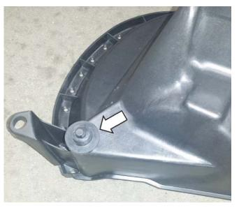
3. Install the rubber isolator into the bottom of the air box (P/N: 131550-9A612).
