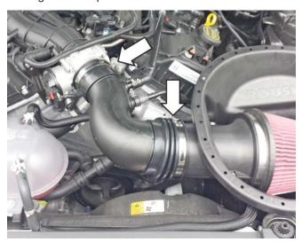
11. Connect the two (2) quick connect fittings previously removed to the new clean air tube.
