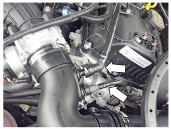
10. Install the clean air tube (P/N: 131537-9R504) and tighten clamps at the throttle body and filter tube. Tighten clamps to 3 Nm.
