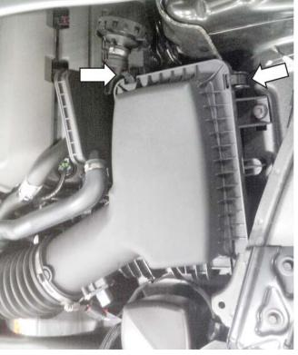
Remove the air box lid and filter. Retain the lid for use during installation.
