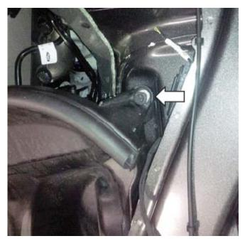
Loosely attach the air filter (P/N: 131550-9601R) to the filter tube (P/N: 131537-12B579), leave the clamp loose so you can hide it once installed in the vehicle.
