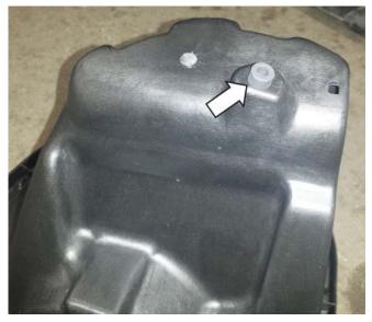
4. Insert the dirty air inlet (P/N: 1315-9F763-A) into the air box (P/N: 131550-9A612).
