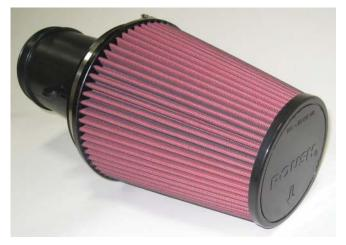
Slide the filter tube assembly into the air box.
