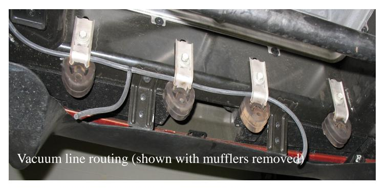
Once all the lines are run, trim any excess. Attach the vacuum lines to each of the exhaust actuators. If using a used exhaust system make sure and debris is cleared for the OEM actuators prior to hooking up the system, give a quick push on the rod to compress the actuator and this should clear them. It's critical that the lines are secured and away from any direct contact with the mufflers. Do not use any clamps or wire ties
