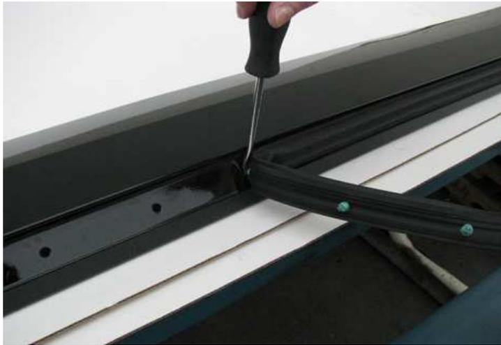
8. Next you need to open the door and get ready to install the door seal on to the Street Scene Side Skirt. You will see all of the holes in line. Drill out with a 3/16 drill bit, then you can install the door seal. See photo below.
