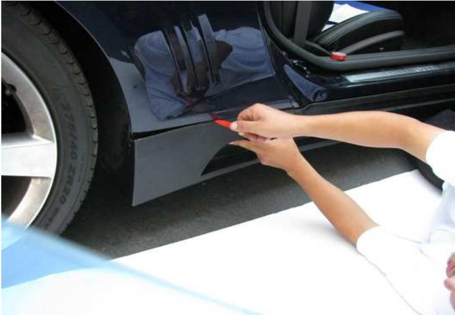
6. After you get the side skirt on in the wheel wells pull around the ends and re-install the two screws in the front and two in the rear of the side skirt.
