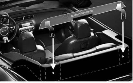
Using the wrench provided, tighten the bolts down on the brackets to secure the windscreen in place.
