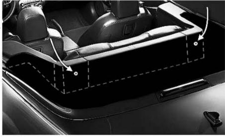
Mount the Windrestrictor by lowering the slotted brackets down on the bolts.
