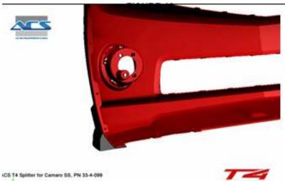
Position the splitter onto the fascia.You may need an assistant's help or clamps to hold in position.
