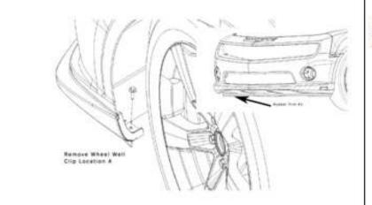
Remove clip located at each extremity of the bumper in front of the front wheel.
