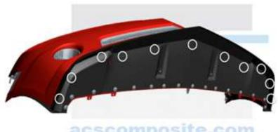
8. Using the Splitter as a template and starting from the centre drill an 8 mm (5/16") diameter holes and install a pressure clip, ensure the fascia and splitter are close together.
