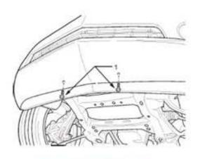
Remove two 10 mm bolts located in the center of the fascia. Save these, as they will be reused to mount the T4 Splitter.
