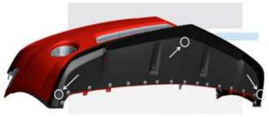
9. Remove M8 bolt from step 7 and reinstall in the circled position. M8 bolt and washers need to be installed at circled positions.
