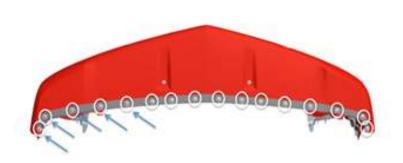
Remove the under carriage rubber seal located at the end of the fascia. Save the clips and seal. These will be reinstalled once the T4 splitter is mounted.
