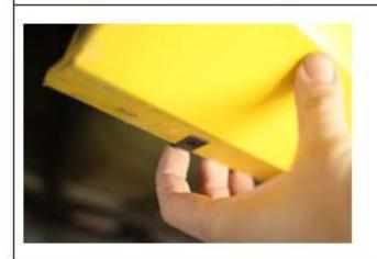
Install the U Nuts by sliding them onto the car's rocker panel from the center of the car towards the outside.
