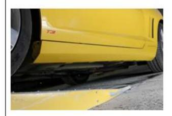
Clean the painted surface of the original rocker on the car. Ensure the underside portion is free of debris and residue. Pay special attention to the rectangular features; shown circled below.
