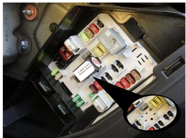
Test by pressing trunk release on the fob (or release button in interior) twice, to open the trunk. Replace panel after verifying operation. That's all there is to it! *Note that the Two-Shot relay remembers the first press indefinitely and will release the trunk on the second press of the button.*
