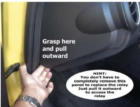
Begin by lifting this panel. Grasp the lower edge and pull outward as shown. There are three spring latches that hold it in place (the two lower ones are easily released, the upper one is difficult). Note that you don't have to completely remove the panel; just pull it out far enough to access the trunk relay. Pull the relay out of its socket and insert the new relay into its place.
