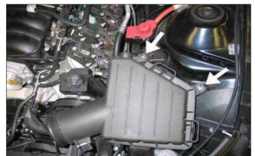
8. Remove the two air box retaining nuts shown.
