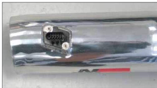
19. Install the mass air sensor into the K&N intake tube and secure with the provided hardware.
