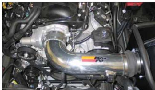
21. Install the K&N intake tube assembly into the silicone hose at the filter adapter and then into the silicone hose at the throttle body and secure with the provided hose clamps.
