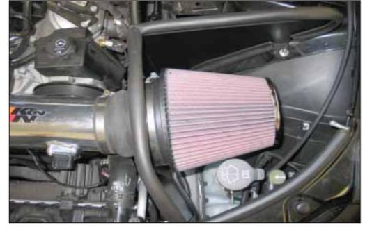
23. Install the K&N air filter onto the filter adapter and secure with the provided hose clamp.
