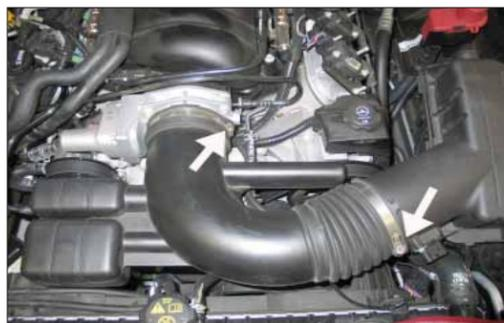
5. Loosen the hose clamps which secure the stock intake tube to the air box and throttle body.
