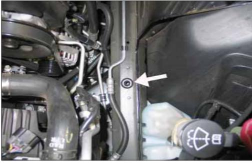
10. Remove the air box mounting grommet shown from the frame rail.
