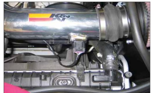
24. Reconnect the mass air sensor electrical connection.
