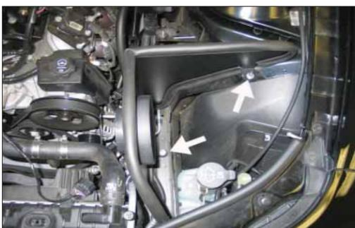
15. Install the heat shield assembly into the vehicle so the inserted nut goes into the air box mounting grommet hole and the tap goes onto the air box mounting stud. Secure the heat shield with the provided hardware.
