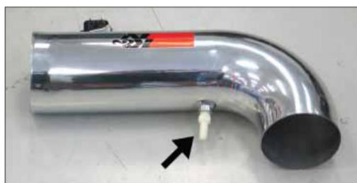
20. Install the provided 1/4npt fitting into the K&N intake tube as shown.
