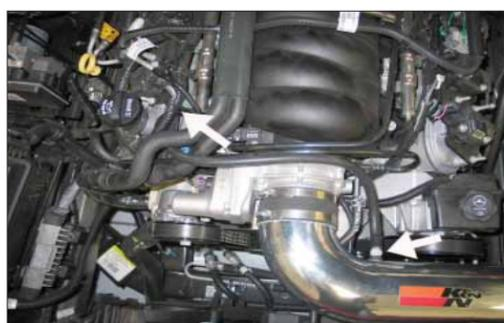
22. Attach the provided crank case vent hose to the 1/4npt fitting and then attach the open end to the vent port on the valve cover.
