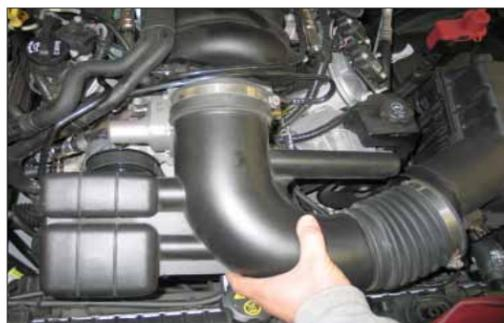
6. Remove the stock intake tube as shown.
