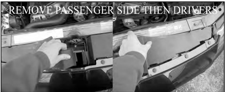
Figure 2. Removal of radiator covers.
