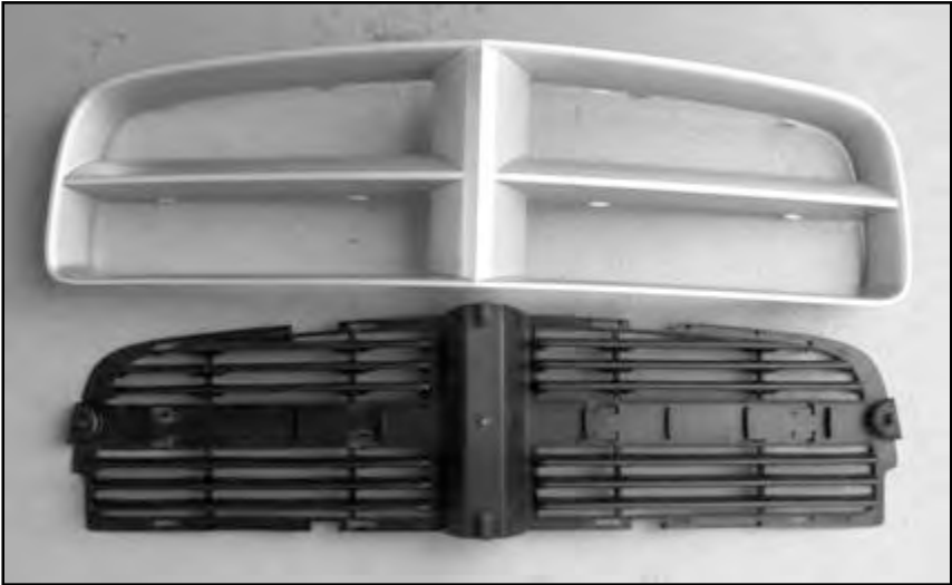
Figure 3. Grille assembly comprising a grille frame (above) and grille.
