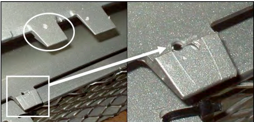
Figure 10. Drill a 1/8" hole on the finished side of the retaining lip. The hole should touch the retaining lip.
