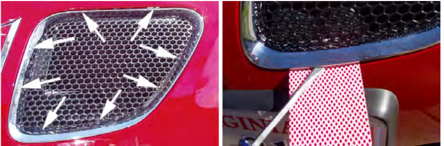
Fig. 1 – Location of upper grille border retainers and method of removal.
