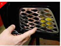
Place the mesh grilles into opening and center. Attach using the supplied  $10-32 \times 5/8$ " bolts. The use of a ball end allen wrench will be necessary as shown above.
