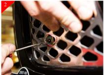
Using a  $90^{\circ}$  scribe mark mounting hole locations. You will be able to reach through one of the marque hole openings to mark locations.
