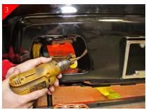
After marking remove mesh grilles from opening. Drill using a 3/16" drill bit as a pilot hole then move to a 3/8" drill bit and drill again as shown. Repeat process for remaining attachment holes. We used a step drill bit, if this method is used take your time and drill to the 3/8" step, do not over drill the hole size.
