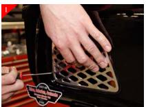
Place the marque mesh billet grille into the bumper opening and center. Check alignment around opening.
