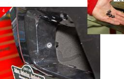
Locate the supplied rubber well nuts (fig. b). Place the rubber well nuts in just drilled locations as shown. Push in place so that the top portion seats against plastic as shown.
