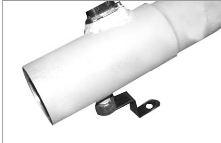
15. Install the provided bracket onto the rubber mounted stud with the provided washer and bolt.
