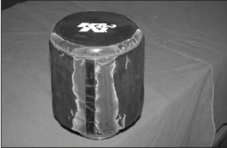
22. Install the K&N Drycharger on the the K&N filter.
