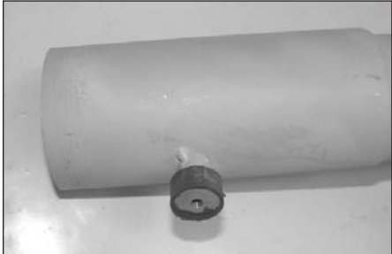
14. Install the provided rubber mounted stud onto the K&N intake tube as shown.
