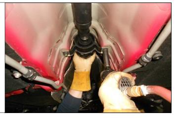
21. The drive shaft can be squeezed together in order to clear the transmission and differential flange.
