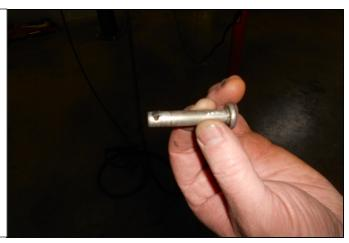
27. Remove the pin on the left and right side by pushing the spring lock down while using a screw driver to pull the pin out until it stops.
