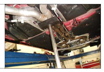
8. Loosen the 15mm nut attaching the left side exhaust flange to the catalytic converter.
