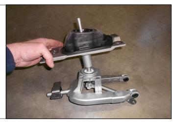
32. Remove the two 4mm allen bolts that hold the factory stick assembly in place.
