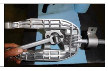
33. Remove the stick assembly from the shifter housing.
