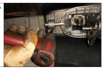
24. Remove the four 15mm bolts from the transmission cross member
