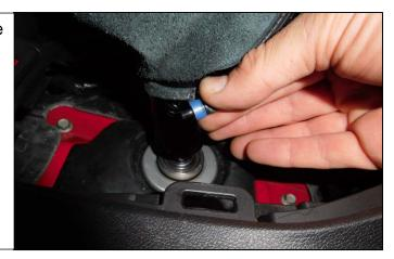
49. Install the shoulder bolts into the pistol grip. Using an 1/8" allen wrench, tighten the shoulder bolts into place.
