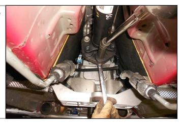
19. Remove the three 18mm bolts and nuts from the flex coupling and differential flange.
