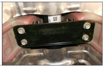
16. Remove the three 10mm bolts from the right and left side of the heat shield. Remove the heat shield.
