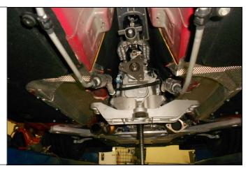
26. The shifter housing is connected to the transmission with a pin on the left and right side. The pin has a spring lock at the end of it as shown here.
