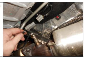
11. Remove the forward rubber isolators from the exhaust system on the left and right side.
