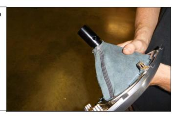
46. Ensure that boot is past the machined groove on the pistol grip and is orientated in the right direction. Secure the shift boot to the pistol grip using the supplied tie wrap.
