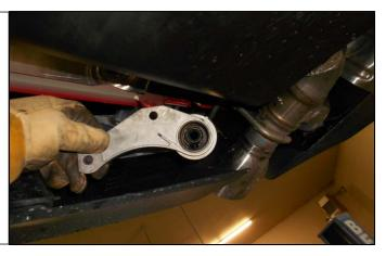
13. The left front exhaust flange is a ball socket you can pry between the transmission cross member and the exhaust to pop it out.
