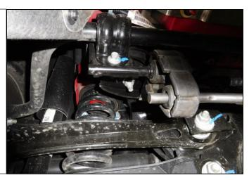
15. Remove the four 13mm bolts from the tunnel brace and remove the brace.
