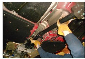
22. Support the transmission with a screw or hydraulic jack.
