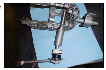
34. Inset all four flange bushings into the supplied link bar. Ensure that the flange portion of the bushing is on the inside of the rod.
