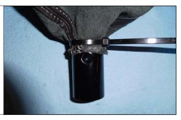
47. Using grease or soap and water, place some lubricant on the O-rings located on the lower stick. With the shift boot still inverted, slide the pistol grip down over the top of the lower stick. Ensure to align the two holes on the pistol grip to the two threaded holes on the lower stick.
