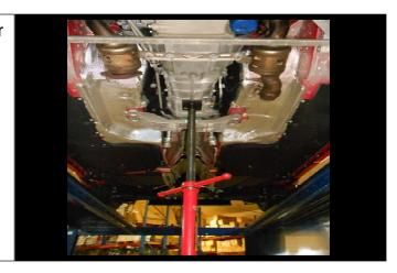
23. Remove the two 10mm bolts from the rear of the shifter housing.
