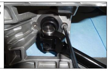
38. Grease the forward bushings on the shift rod and reinstall the factory rubber boot.
