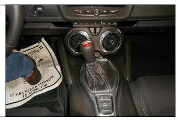
2. Using a trim tool, pry up on the back of the chrome bezel.
