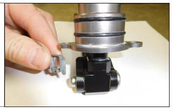
37. Insert the Hurst shifter assembly into the factory housing. Install the supplied bolts. Bolt it in place using a 4mm allen wrench.
