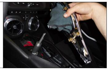
5. Using an extension and 10mm socket, remove the 4 bolts attaching the rubber boot to the transmission tunnel.
