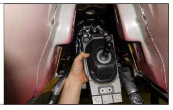
40. Reinstall the two spring pins that attach the shifter housing to the transmission.
