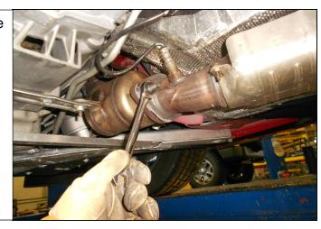
10. Unplug the oxygen sensor that is attached to the right side exhaust. Make sure it is free and clear.
