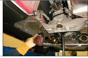
25. Lower the rear of the transmission enough to gain access to the front of the shifter housing.
