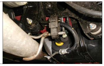
12. At the rear of the vehicle there are two mounted hangers located on the left and right side. Remove the two 15mm nuts that attach each hanger then remove the hangers.
