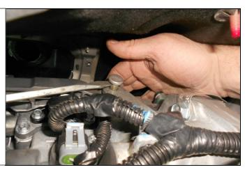
**Note:** The pin can be rolled to gain access to the spring lock.
