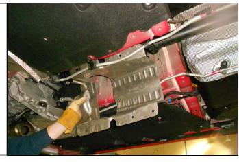
17. The drive shaft must be removed. Start by making an alignment mark on the flex coupling and the transmission flange.
