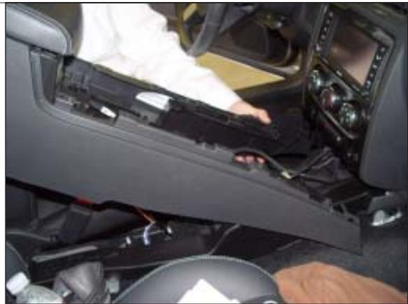
**STEP 11.** Remove rear A/C duct by pulling rear ward.
