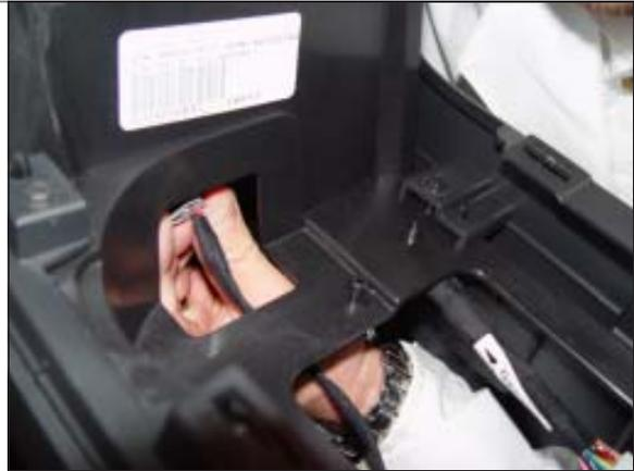
**STEP 10.** Slide rearward or remove the center console to gain access to the shifter.
