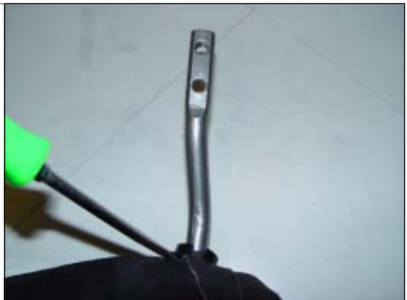
**STEP 38 (optional).** Install the leather boot onto the boot support using the supplied tie wrap (trim away excess tie) and snap boot bezel into center console.
