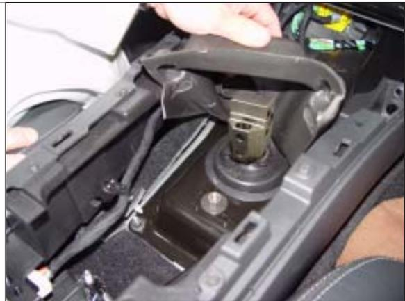
**STEP 26.** Install the rear A/C duct.
