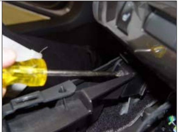
**STEP 7.** Remove the rubber tray in the center console storage box.
