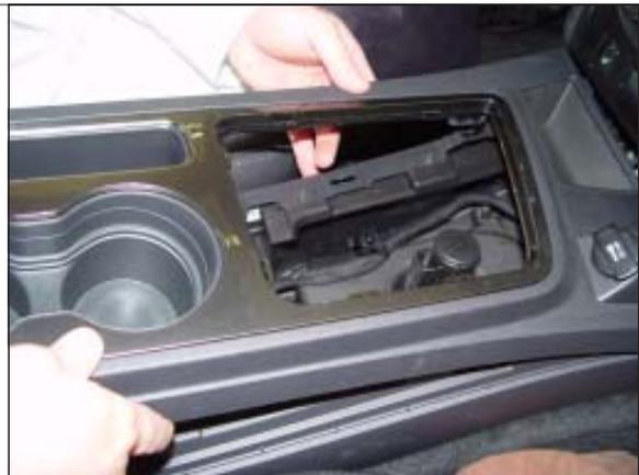
**STEP 35.** Bolt in the upper stick assembly on to the Hurst Shifter and torque to 20Nm (15 ft-lbs).
