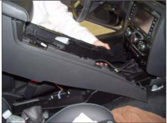
**STEP 28.** Raise the center console to access and reconnect the center console storage box lighting connection and any additional wiring connection clips.
