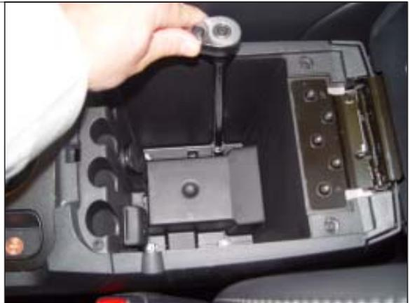
**STEP 30.** Replace the rubber tray in the center console storage box.
