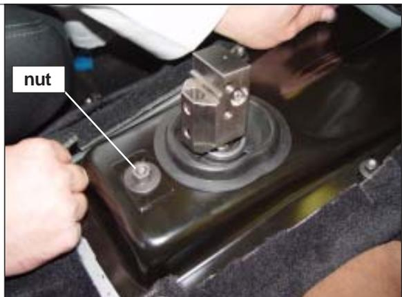
**STEP 23.** Install the six tunnel cover mounting nuts and torque to 20 Nm (15ft-lbs).
