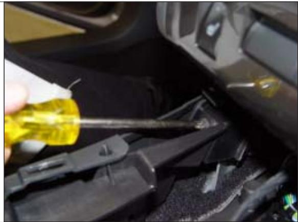
**STEP 32.** Reconnect the cupholder lighting connection under the center console trim/cupholder plate.
