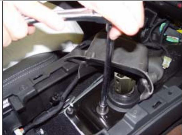
**STEP 25.** Install the rubber shift boot cover and the wiring routing ties.
