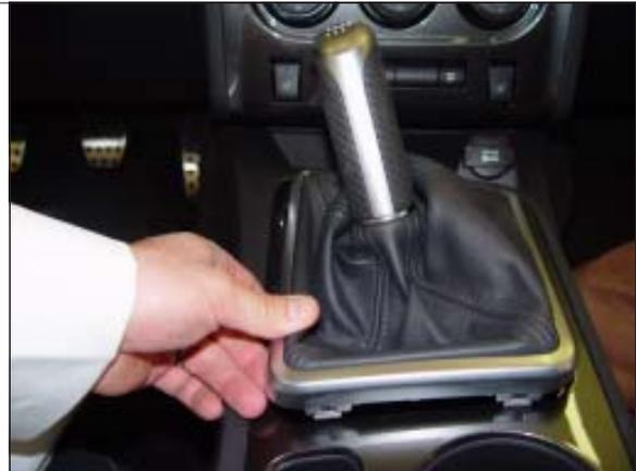
**STEP 2.** Unbolt the upper stick assembly from the shifter and remove knob, boot, stick assembly.
