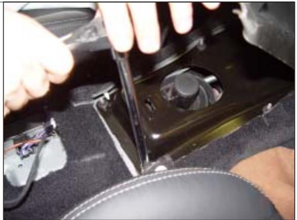
**STEP 15.** Detach shifter boot from metal tunnel cover and remove cover.
