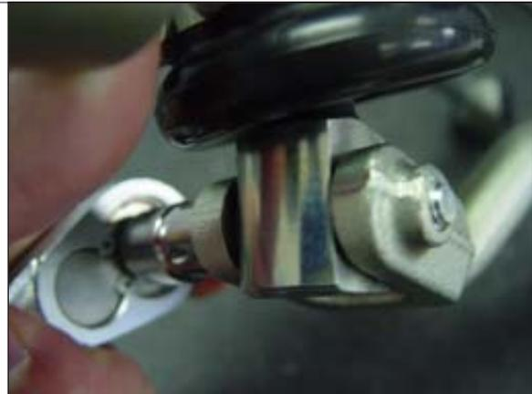
**STEP 18.** Carefully remove both the upper and lower rubber shifter boots from the assembly. Avoid ripping or tearing the boots. If they are damaged, contact your local Dodge dealer for replacements.
