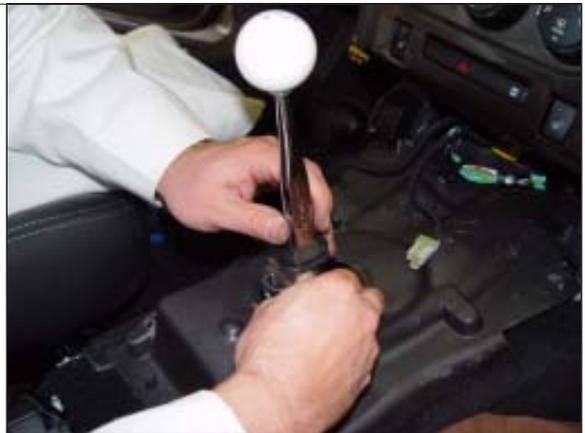
**STEP 38 (optional).** Disassemble leather boot from stock stick/knob/boot assembly by prying open the boot clip and removing leather boot.
