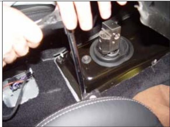
**STEP 24.** Tighten the rear mounting nut and torque to 20 Nm (15 ft-lbs).
