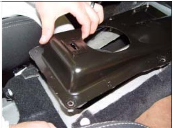
**STEP 16.** Unclip and pull out the two front lock pins that hold the shifter bracket to the transmission.
