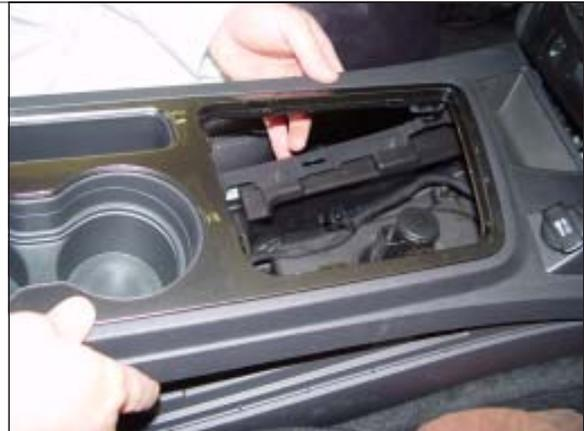
**STEP 4.** Disconnect the 12V accessory/cigarette lighter socket wiring harness connection.
