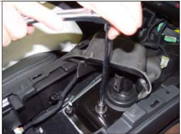
**STEP 14.** Unscrew six tunnel cover mounting nuts.
