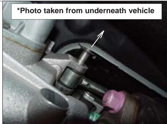
**STEP 17.** From inside the vehicle, lift up on the shifter assembly to access the lower change rod connection bolt and remove both bolt and then shifter from vehicle.
