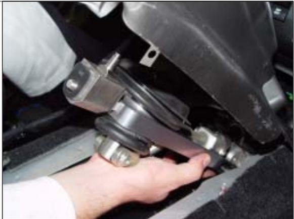
**STEP 21.** Position Hurst Shifter into vehicle and install and lock front pins.
