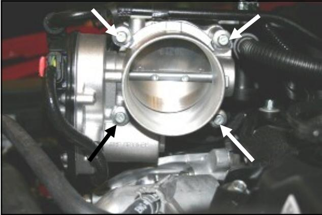
3. Remove the four bolts that secure the throttlebody to the intake manifold and set aside. They will not be reused.
