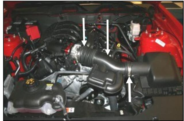
6. Reinstall the intake tube, tighten the two hose clamps, and reconnect the breather line or lines.
