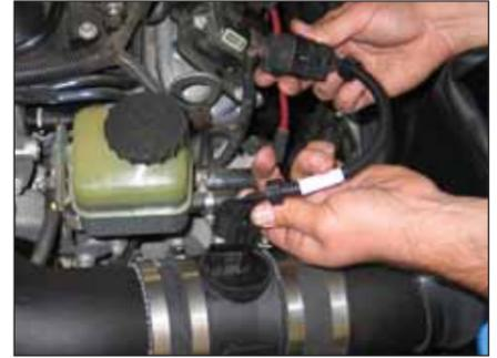
22. Connect the provided mass air sensor extension harness to the factory connector and then to the mass air sensor as shown. Route the wiring harness behind the mass air sensor for clearance from the engine cover.
