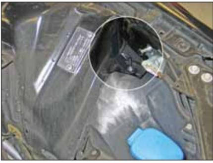
10. Install the heat shield mounting bracket (07190) onto the air box mounting stud using the provided hardware.
