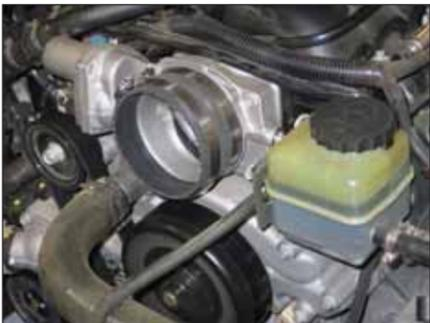
14. Install the silicone hose (08618) onto the throttle body and secure with the provided hose clamp.
