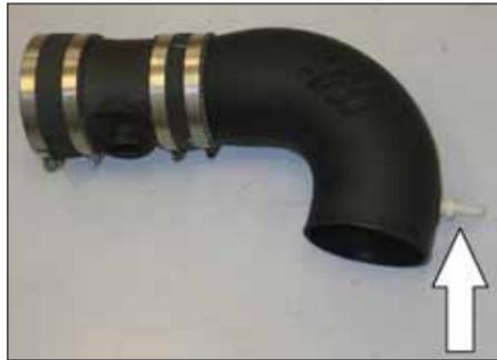
20. Install the crankcase fitting into the K&N® intake tube as shown.
