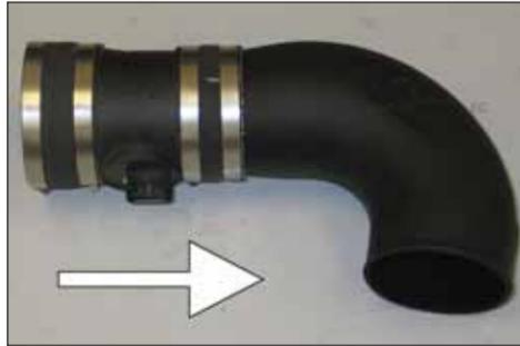
19. Install the mass air sensor assembly onto the K&N® intake tube as shown.
