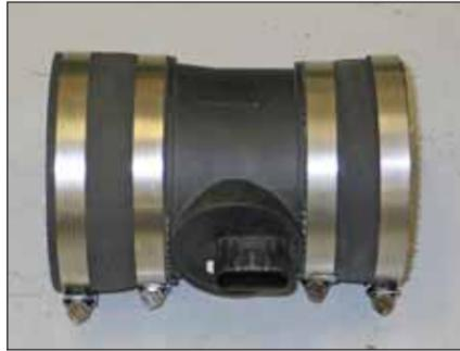
17. Install the provided silicone hose (08536) onto the mass air sensor and secure with the provided hose clamp.
