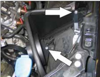
13. Install the heat shield assembly into the vehicle and secure it to the mounting bracket installed in step #10 and to the air box mounting stud location.
