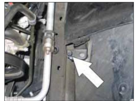
9. Remove the air box mounting stud shown.
