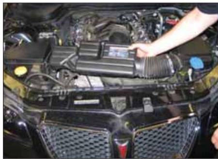
5. Remove the complete stock intake tube assembly from the vehicle as shown.
