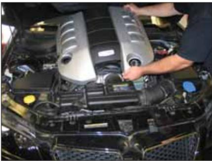
2. Remove the oil fill cap and then remove the engine cover from the engine as shown. Reinstall the oil fill cap.
