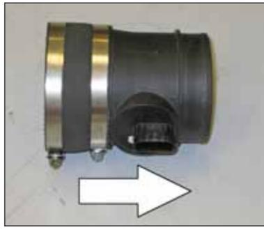
16. Loosen the hose clamp and remove the mass air sensor from the factory air box. Install the provided silicone hose (08761) onto the mass air sensor and secure with the provided hose clamp.
