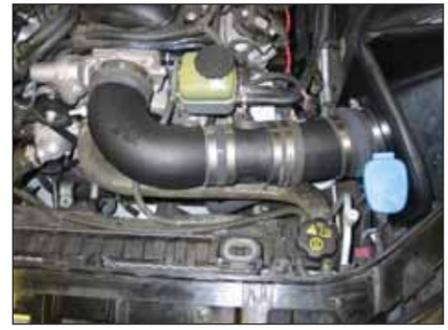
21. Install the K&N® intake tube with mass air sensor into the silicone hose at the throttle body and onto the intake tube on the filter adapter. Rotate and adjust the intake tubes for proper fit and then secure the assembly with the hose clamps.
