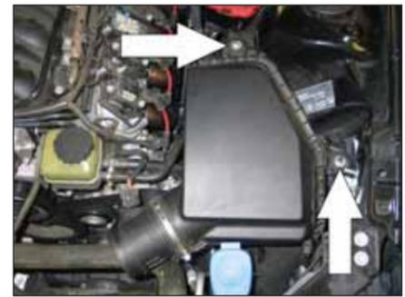
7. Remove the two air box mounting nuts shown.
