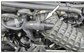
4. Release the spring clamp securing the sound tube to the fitting in the intake tube and then disconnect the sound tube.
