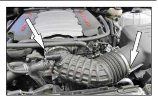
5. Loosen the hose clamps securing the intake tube to the throttle body and air filter housing and then remove the intake tube.
