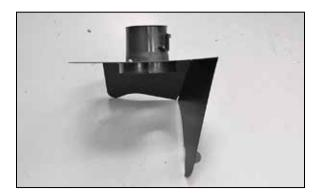
13. Install the K&N® mass air sensor housing into the heat shield and secure with the provided hardware.
