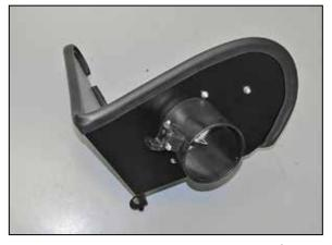
19. Install the mass air sensor into the  $K\&N^{\otimes}$  mass air housing and secure with the provided hardware.
