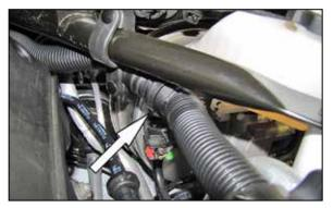
9. Disconnect the sound tube quick disconnect fitting and remove the complete sound tube system.
