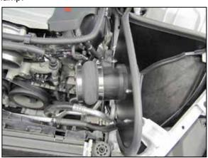
22. Install the provided step hump coupler (08695) onto the filter adapter and secure with the provided hose clamp.
