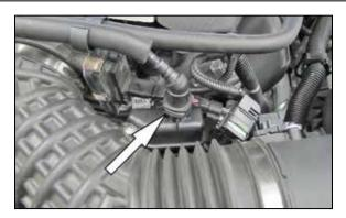
3. Disconnect the crank case vent quick connect fitting from the intake tube.
