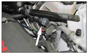
11. Install the cap assembly into the remaining sound tube.
