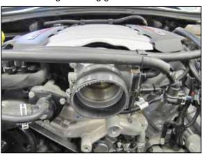
21. Install the provided coupler hose (08761) onto the throttle body and secure with the provided hose clamp.
