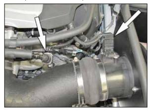
26. Connect the crank case vent hose to the quick disconnect fitting installed into the K&N® intake tube. Connect the mass air sensor electrical connection.
