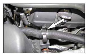
7. Open the clamp securing the sound tube to the air filter housing.
