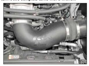
25. Install the K&N® intake tube into the hump coupler and then into the coupler at the throttle body, adjust the tube for best fit and then secure with the provided hose clamps.
