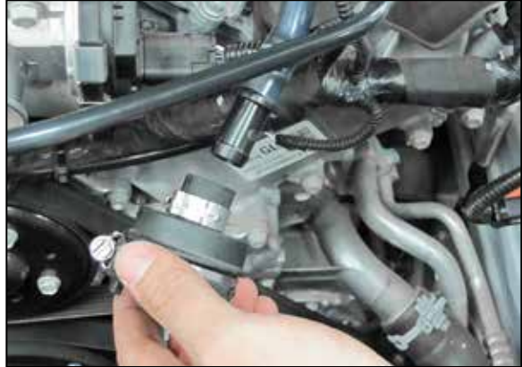
11. Remove the factory crank case vent coupler from the crank case vent tube. NOTE: Us twisting/pulling motions to slip the coupler off the tube, it is not necessary to cut the factory clamp.
