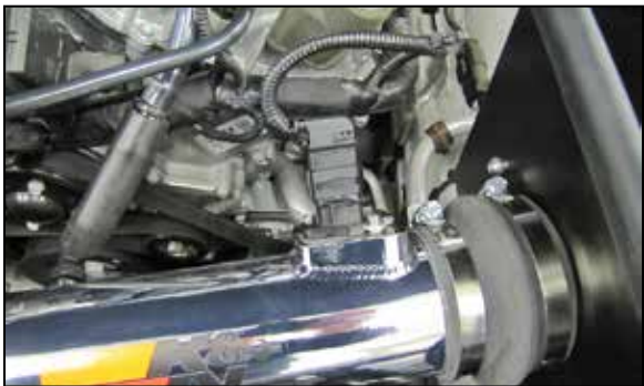
27. Reconnect the mass air sensor electrical connection.
