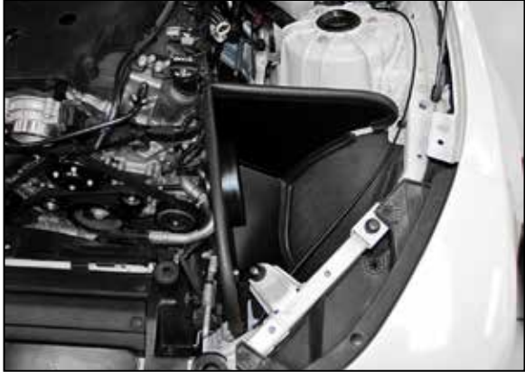
16. Install the heat shield assembly onto the factory air filter housing mounting grommets.
