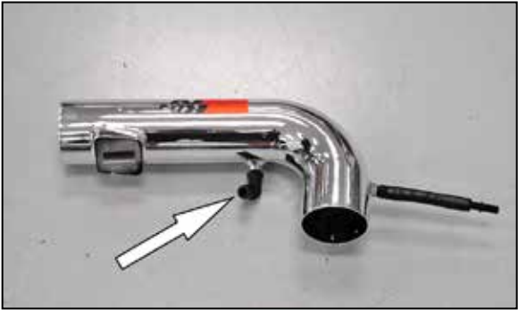
21. Install the 90° crank case vent fitting into the K&N intake tube as shown. NOTE: Plastic NPT fittings are easy to cross thread. Install the vent fitting “hand” tight, then turn it two complete turns with a wrench.
