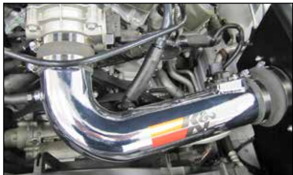
26. Install the provided crank case vent hose onto the factory vent hose and K&N® fitting.
