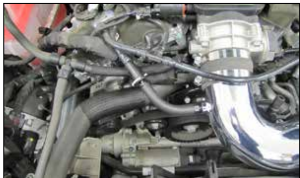
25. Connect the K&N® EVAP quick disconnect fitting into the factory fitting.
