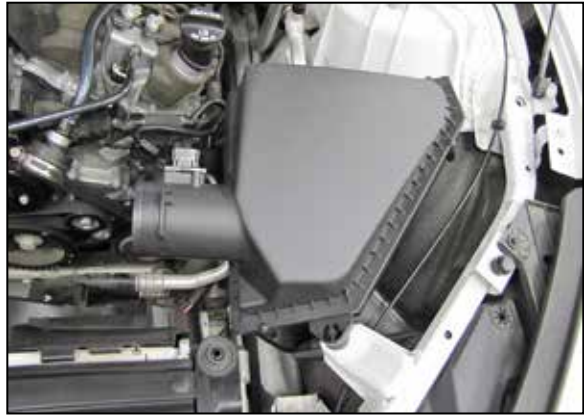
10. Lift up and remove the factory air filter housing assembly. NOTE: K&N Engineering, Inc., recommends that customers do not discard factory air intake.
