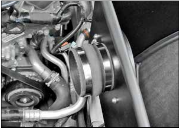
18. Install the provided hump coupler (084079) onto the filter adapter and secure with the provided hose clamp.
