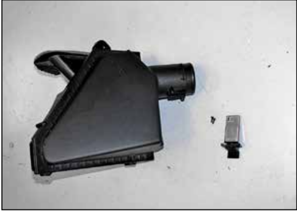
22. Remove the mass air sensor from the factory air filter housing.
