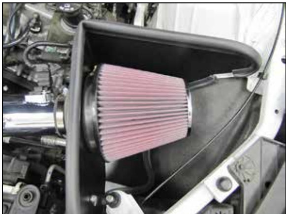
28. Install the K&N® air filter and secure with the provided hose clamp.
