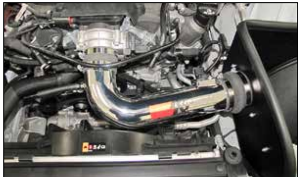
24. Install the K&N® intake tube assembly into the coupler at the filter adapter and then into the coupler on the throttle body, adjust the tube for best fit and then secure with the provided hose clamps.
