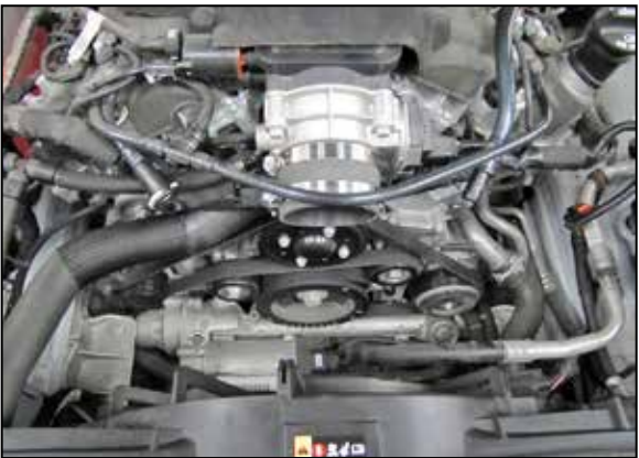
17. Install the provided coupler (084031) onto the throttle body and secure with the provided hose clamp.
