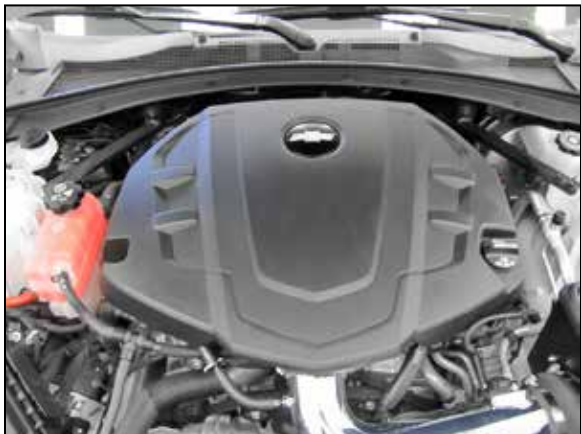
29. Reinstall the decorative engine cover and secure with the factory bolt and oil cap.
