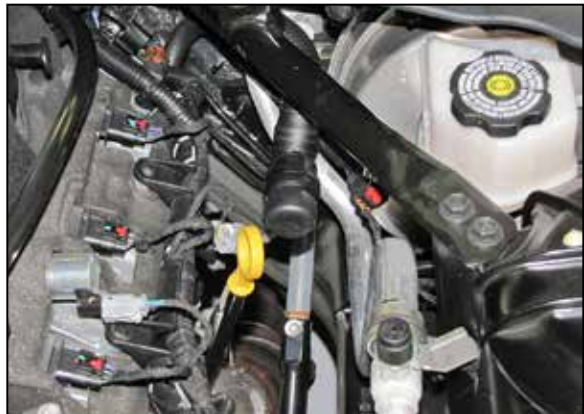
8. Install the capplug assembly into the remaining sound tube and secure with the provided tie wrap.
