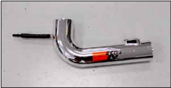
20. Install the EVAP hose assembly onto the K&N intake tube as shown.
