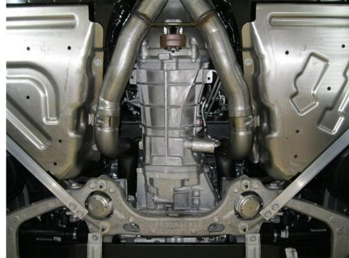
**Step 3.** Next Loosely attach the Muffler Assemblies to Inlet pipe using the provided 3.00" clamps. You will then need to fasten the provided cross bracket in place between the two muffler assemblies using the provided 1/4" fasteners. Insert all hangers in the rubber insulators.
