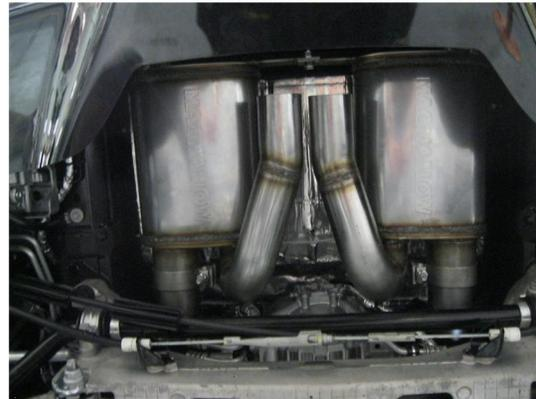
**Step 4.** Now you can re-attach the rear valance to the vehicle using the OEM fasteners. Once the rear valance is back in place loosely attach the Tip assembly to the Muffler assemblies using the provided 2.50" clamps.
