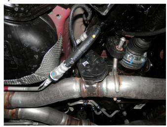
**Step 2.** Next you will need to unplug the electrical connection on the Exhaust Valve Control Motors (Qty 4) located on the OEM exhaust assembly.
