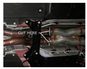
**Step 1.** It is necessary to cut the factory exhaust system to install the new Magnaflow unit. To do this cut the band clamps holding the heat shield to the pipes in front of the X. Move the heatshield out of the way and cut 1/2" in front of the welds on the factory X-Pipe. Deburr the cut pipes to facilitate installation of the new system.
