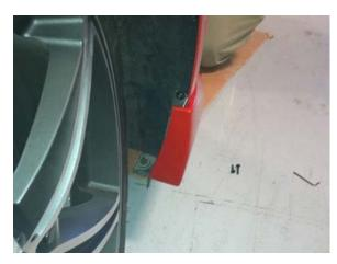
3. Prior to drilling the holes in the front air dam and bracket, measure the distance from the bottom of the side marker to the top of the front air dam on both the passenger side and driver side of the car to make sure they are even. Drill two holes into the back of the air dam where it meets the bracket for mounting. Repeat on driver's side
