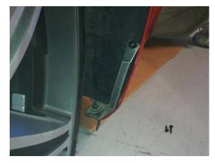
2. Fit the UNPAINTED front air dam over the front fascia starting from the driver's side wheel well and working over to the passenger side wheel well. You may want to use some painters tape over your front fascia during the test fits to protect your paint.
