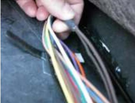
**STEP 6:** Use the provided wire tap clamp and place one end of the positive red wire coming off of your WR light into the inner part of the clamp until it stops, then hold it in place firmly. Insert the desired wire (Blue or Darkest Brown) through the outer edge of the wire tap clamp and while holding both wires in place, squeeze the clamp so that it is tight and both wires are secure.
