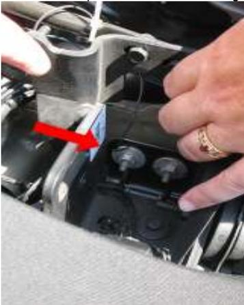
**STEP 3:** Locate the rubber grommet on the passenger side of the rear quarter panel in the trunk and unscrew it and the nut behind it.
