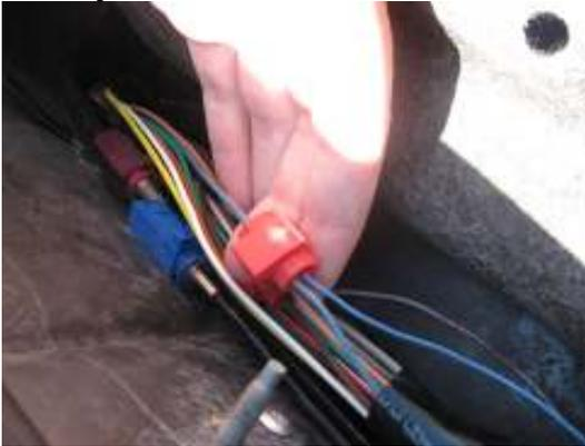
**STEP 7:** Check and make sure that your LED strip for the WR lights up correctly by turning on your headlights or stepping on the brakes. Remember that in the Sky and Solstice, if your car is not running the brake lights will not come on, so you may need to start your car to check this.
