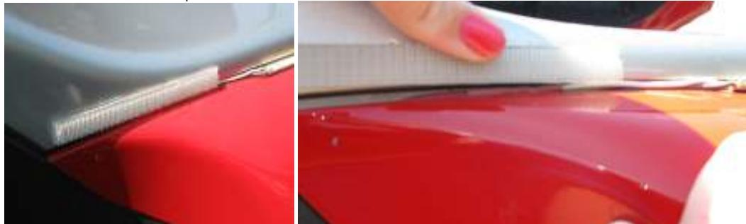
**STEP 10:** Place Wind Restrictor on top of console where it will be mounted, but do not stick it to the panel yet... Make sure Wind Restrictor is evenly spaced and balanced paying attention to where the LED light strip will need to go.
