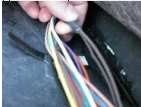
**STEP 7:** Use the provided wire tap clamp and place one end of the positive red wire coming off of your WR light into the inner part of the clamp until it stops, then hold it in place firmly. Insert the desired wire (Blue or Darkest Brown) through the outer edge of the wire tap clamp and while holding both wires in place, squeeze the clamp so that it is tight and both wires are secure.
