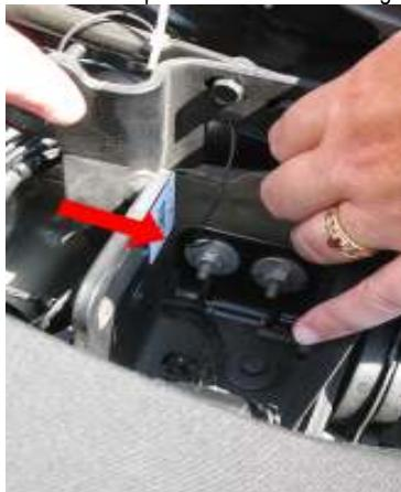
**STEP 4:** Locate the rubber grommet on the passenger side of the rear quarter panel in the trunk and unscrew it and the nut behind it.
