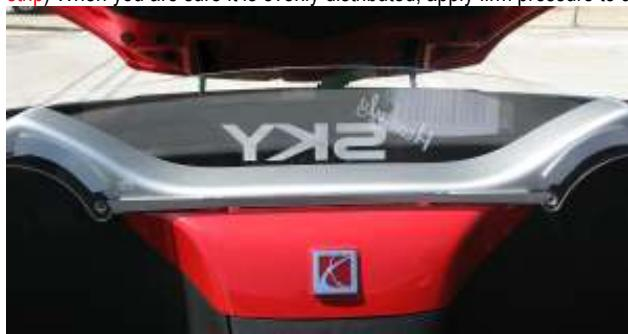
**STEP 14:** Push both seats all the way back resting on the WR and allow them to keep pressure on it for at least 72 hours to make sure that the adhesive has had time to cure to the silver panel of your car.
