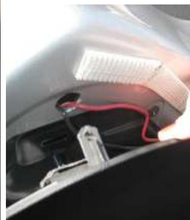
**STEP 3:** Unscrew the nut shown in the photo so that you can ground the black wire behind it. Once it is loose, place the circle ground clamp that you have attached to the black wire provided in the tackle bag over the post. Now tighten the nut securely back in place, making **a good ground connection**.
