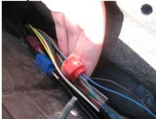
**STEP 8:** Check and make sure that your LED strip for the WR lights up correctly by turning on your headlights or stepping on the brakes. Remember that in the Sky and Solstice, if your car is not running the brake lights will not come on, so you may need to start your car to check this.
